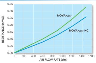
Test data results based on 24" x 24" x 1" filter sample.
